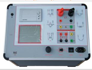
Model CPT1200 CT PT ANALYZER is mainly used for field testing of P class CT and PT. The test items mainly include excitation characteristic, transformation ratio, polarity, Degauss, 5% and 10% error curves, secondary circuit check, withstand test of power frequency alternating current and secondary load. Adopt LCD, self-equipped minitype printer supporting field printing; supporting to use USB flash disk to dump data, with simple and convenient operation.
